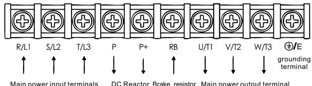
18.5KW-355KW (380V) Main Circuit Terminals (Left input right output)
