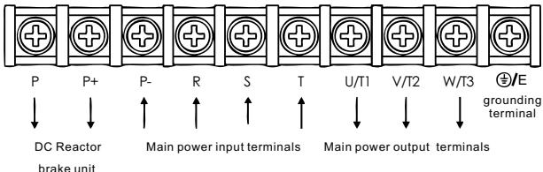
45KW-250KW (380V) Main Circuit Terminals (Up input down output)
