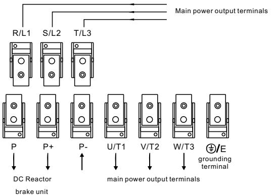
Note: P/P+ Standard setting is short circuit; if it is with external Dc Reactor , please disconnect and then connect it.
